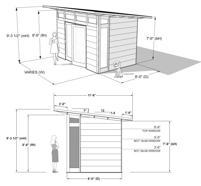
(D) = SHED DEPTH | (W) = SHED WIDTH | (mH) = MAX ROOF HEIGHT | (fH) = FRONT WALL HEIGHT | (bH) = BACK WALL HEIGHT
